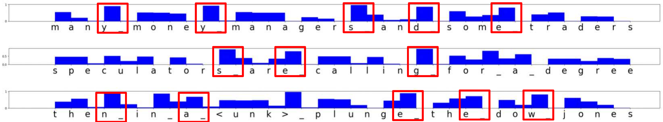
Figure 4: Syntactic distance estimated by Parsing Network. The model is trained on PTB dataset at the character level. Each blue bar is positioned between two characters, and represents the syntactic distance between them. From these distances we can infer a tree structure according to Section 4.2.
